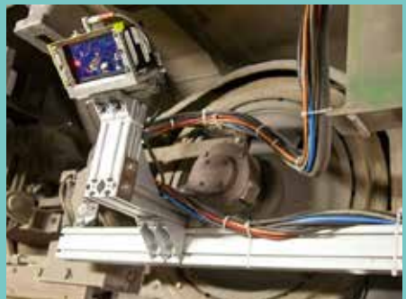
Yarra Trams – video cameras and laser scanners capturing data of the tracks
